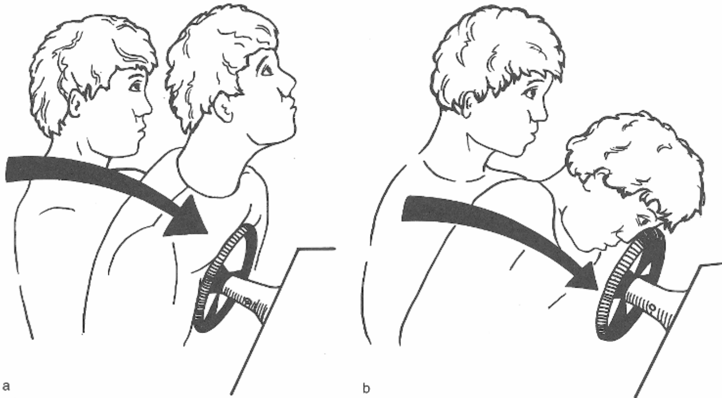
Figure 8.9 (a) Unrestrained driver thrown chest first into the steering column. (b) The torso of a driver restrained by a lap seat belt rotates forward and results in head impact with the steering wheel assembly.
